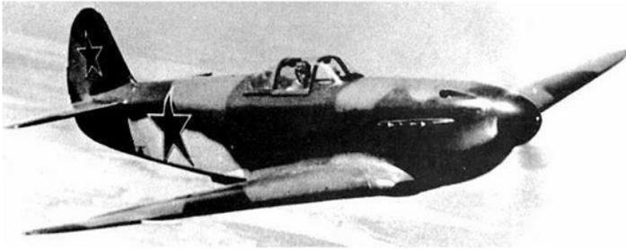
The Yak 3 was a highly maneuverable, low-altitude fighter-interceptor. All German pilots were taught to fear the Yakovlev 3 because it could outturn, out-climb and out-accelerate both the Messerschmitt Bf 109 and Focke-Wulf 190s at the low altitudes at which it tended to operate.
